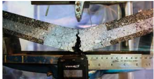
An unreinforced asphalt pavement beam with a conventional tack coat predictably cracks under stress in a short period of time.
